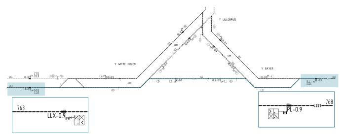
At 12.27 p.m., the drivers of the two trains realised that they were traveling towards each other on the same track 763 and they responded. After braking, their trains were 200 meters apart.
