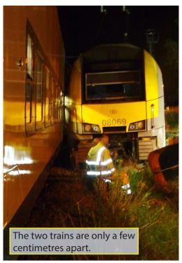
The first contributing factor is that due to the lack of attention to the shunting movement, the train driver does not see the buffer stop with marker board at the end of the dead-end track 091, causing him to neither slow down nor brake.
