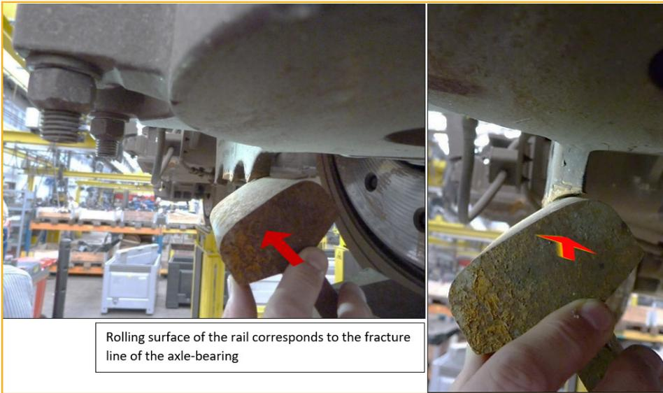
Rolling surface of the rail corresponds to the fracture line of the axle-bearing
