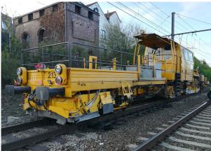
While crossing this switch, the first axle of the ballast regulator derails at low speed. The driver, having felt the shocks, brakes immediately. The ballast regulator stops on the switch, encroaching on the loading gauge of both tracks.
