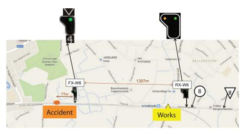
The driver encounters 9 consecutive green flashing signals. Then he encounters a green-yellow horizontal flashing warning signal (RX-W.6) that informs him of the aspect of the following signal (FX-W.6). In the absence of a speed indication (on the signal RX-W6) the train is permitted to travel at a restricted speed of 40km/h from the next dangerous point.
