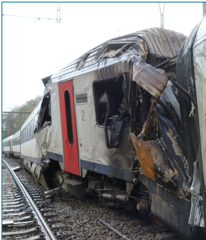
The front of the first railcar of the AM449, with the traces of the fire, collided with the train E940 in Bracquegnies.
