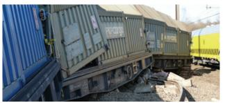
At 16:43, the train driver called Traffic Control and signalled that the train was stopped at the entrance signal to the Muizen sidings and that the brake circuit was depressurised, wagons 14 to 19 of the freight train E47582 had derailed on the track change AW 03U at the Hever branch. A broken axle coming from the first derailed wagon was found at the place of derailment.
