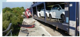
The first train, E47540, was made up of 20 wagons filled with scrap metal. Some of the wagons suffered an impact in the collision but were not derailed. The second train, Z65292, was made up of 19 wagons transporting cars. Several wagons derailed and one of them fell to the bottom of the Galoppe viaduct. Train traffic was suspended in both directions of line 24 for around 18 hours.
